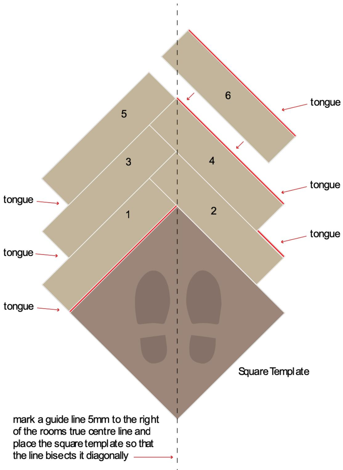
mark a guide line 5mm to the right of the rooms true centre line and place the square template so that the line bisects it diagonally
